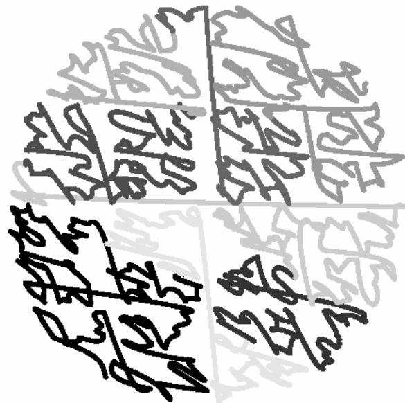
FIG. 1. The self-similar space filling curve (Morton order) connecting the particles which is used to obtain the domain decomposition. Eight processor domains are shown in different levels of gray.
